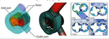
The essence of our original technologies behind abundant track record, is concentrated into profiling Air Block. The 3-D fluid analysis that makes full use of an advanced CFD (Computational Fluid Dynamics) technology simulates to assist in optimising shapes of air flow path, inlet, outlet and rotor.
