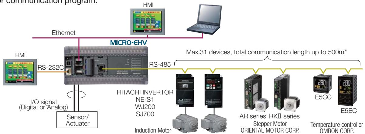
\* In case of combine with stepper motor by ORIENTAL MOTOR CORP., total communication length is up to 50m
