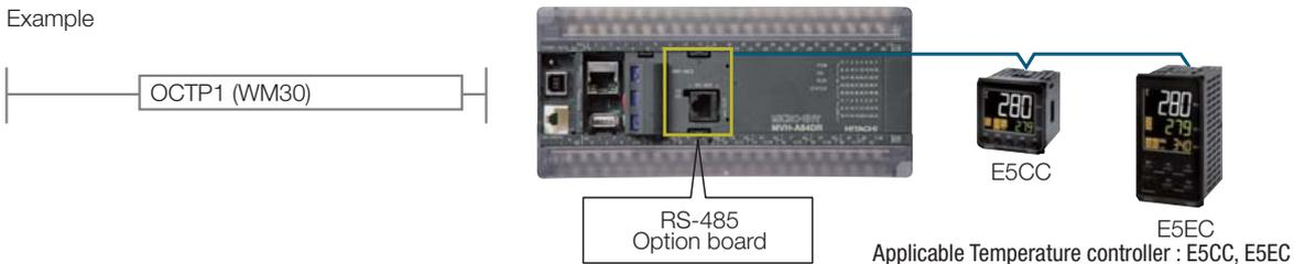
"OCTP1" command is dedicated command of control and monitoring for OMRON's temperature controller. (Applicable temperature controller : E5CC, E5EC)
